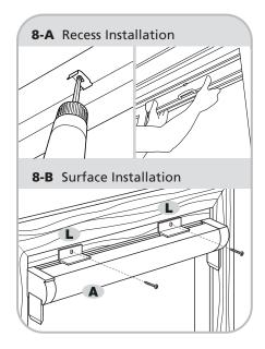
NOTE: It is critical that the Screen Cassette and Rails be installed square and plumb in the door opening. Apply shims (not supplied) as needed.
