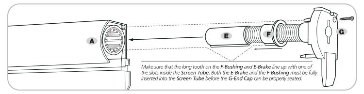
Slip the F-Bushing down the coiled spring to the E-Brake. On the open end of the A-Screen Cassette, insert the E-Brake with F-Bushing into the center of the Screen Tube, aligning the long tooth on both as noted above. Next, match up the large pin on the top of the G-End Cap to the corresponding hole at the top of the A-Screen Cassette Housing. Tap evenly with a soft mallet until the assembly fits snugly.
