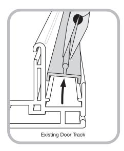
If however, the existing door's Screen Track is removable, take out the Track by hand or with any type of pliers [E2].
