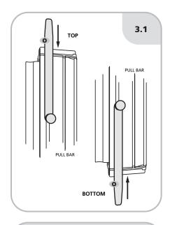
**OPTIONAL** • INSTALLING THE SLIDE BOLT ACCESSORY LOCK
