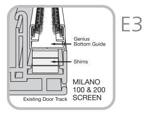
Then add non-degradable shim material (plastic, nylon or similar) [E3] to create a flat and stable surface for the Milano 100 or 200 Retractable Screen Bottom Guide Rail.
