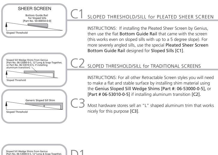
Sloped Sill Wedge Shims from Genius [Part No. 06-53000-0-5, 12"Long & Snap-Together, or Part No. 06-53010-0-5, if installing aluminum transition] Sloped Threshold Original Existing Screen Track
